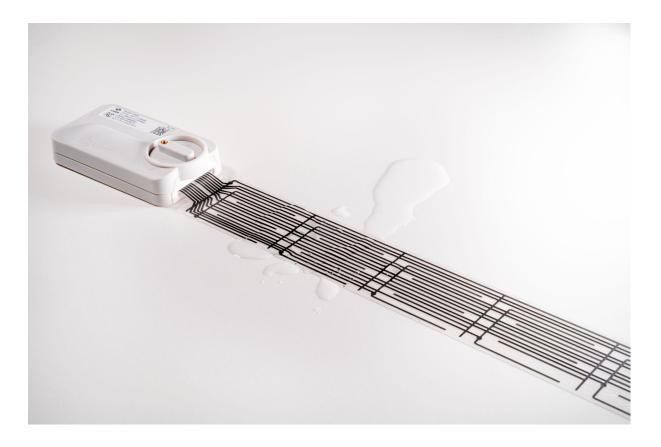
Severn WLD is LAIIER's water leak detection device. The Severn WLD hardware connects to a printed sensor that is split into 12 sections or electrodes. Upon powering up with a single AA Li-SOCI2 cell battery, the device connects to the LoRaWAN® network via OTAA. After running through a self-test, the device enters its run mode.
