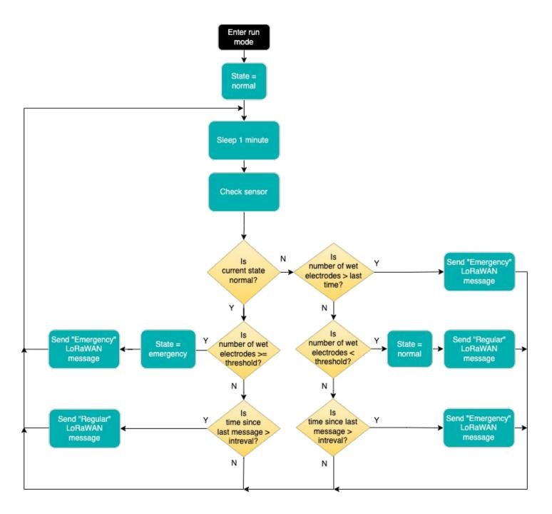
When the device enters run mode, its state is set to normal, and it checks for the presence of water on each electrode every minute (please review <u>Electrode definition and sensor dimensions</u> to clarify what an electrode is). By default, 4 electrodes need to be wet for the device to sense a leak.
