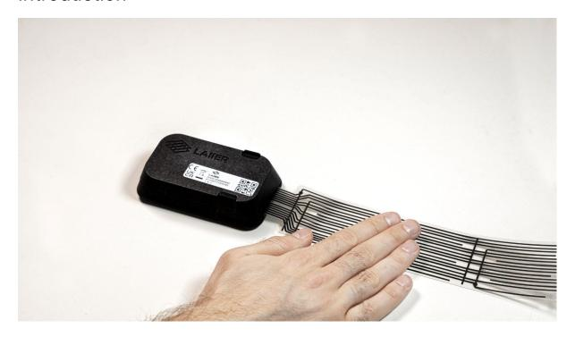
Severn WLD is LAIIER's water leak detection device. It consists of a printed sensor that is split into 12 sections or electrodes, which gets connected to the Severn WLD hardware. Upon powering up with a single AA Li-SOCI2 cell battery, the device connects to the LoRaWAN® network via OTAA. After running through a self-test, the device enters its run mode.
